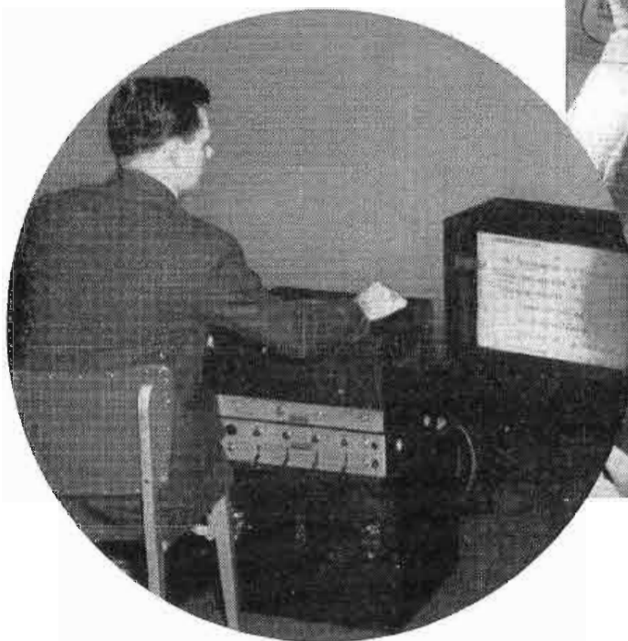
A Teleprompter user, reading his speech as it unrolls before him, is able to make his delivery sound extemporaneous. At left: An operator in the wings, working from an identical typewritten version of the text, adjusts the speed of the Teleprompter to the vocal speed of the speaker.
